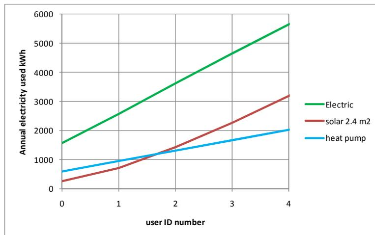
Fig. 8. Annual electricity used by three water heating options: reference electric, a solar and heat pump in the North zone.
