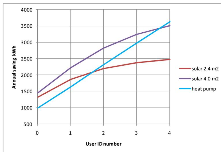
Fig. 9. Annual savings achieved (in kWh) by two solar options and the heat pump water heater in the North zone.
