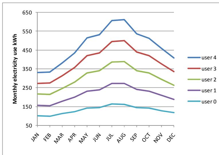
Figure A2 Monthly electricity use by the reference electric water heater for zone 5
