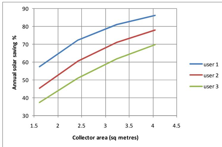
Fig. 11. Influence of evacuated tube solar collector area on the annual electricity saving in the North zone.
