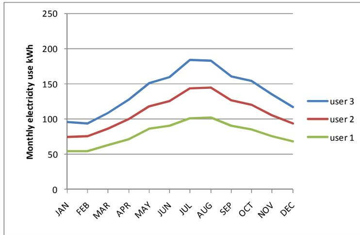
Fig. 7. Monthly electricity used by the representative heat pump water heater in the North zone.
