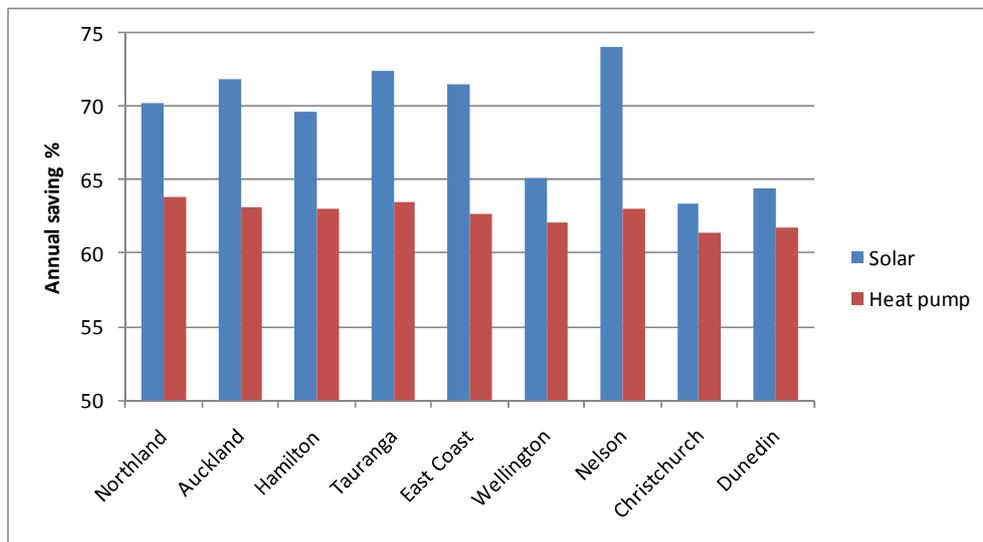
Fig. 15. Annual electricity saving for a medium user with solar and heat pump water heaters. For all centres the collector area 3.2 m<sup>2</sup> except for Dunedin where the collector area is 4.0 m<sup>2</sup>.
