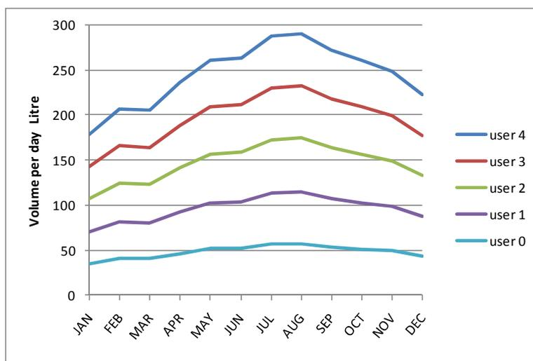
Figure A3 Daily volume of hot water use for the reference electric water heater for zone 5
