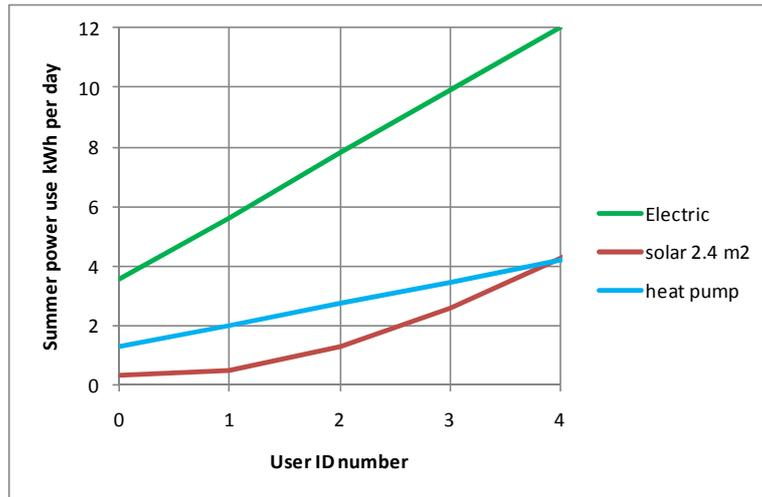
Fig. 17. Average electricity use per day during the summer months December – March by three water heating options: reference electric, solar and heat pump in the North zone.
