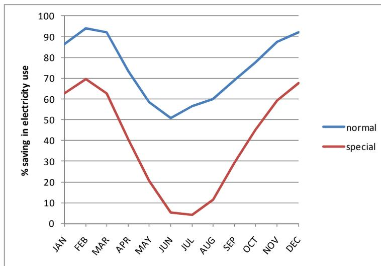
Fig. 21. Influence of adverse control on the annual saving in electricity use by a solar water heater with collector area 2.4 m<sup>2</sup> (30 evacuated-tubes).in the North zone. For the curve labelled “special” the electric booster element and thermostat were located near the bottom of the tank.
