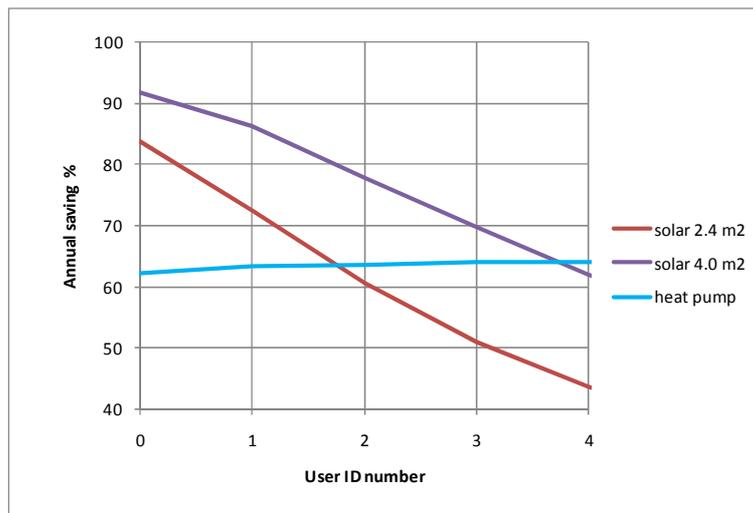
Fig. 10. Annual savings achieved by two solar options and the heat pump water heater in the North zone expressed as a percentage of the reference electric water heater use.
