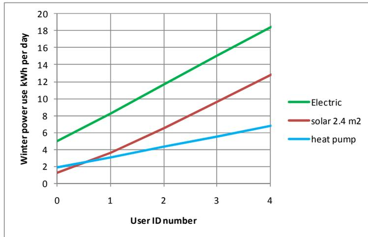
Fig. 16. Average electricity use per day during the winter months May – August by three water heating options: reference electric, solar and heat pump in the North zone.
