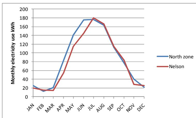
Fig. 13. Monthly electricity demand for a consumer with a solar water heater in Nelson compared with one in Auckland. The user has a medium demand and the solar collector area is 3.2 m<sup>2</sup> (40 evacuated-tubes)
