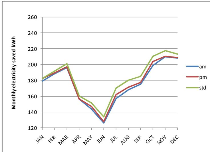
Fig. 1. Effect of different daily water use profiles on the saving in monthly purchased electricity for a medium level user in the North zone using a 2.4 m<sup>2</sup> solar collector (30 evacuated-tubes).
