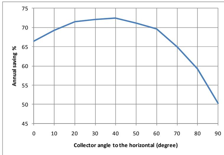
Fig. 20. Effect of the collector angle to the horizontal on the annual electricity saving for a solar collector area 2.4 m<sup>2</sup> (30 evacuated-tubes) for user-1 in the North zone.
