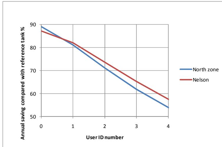
Fig. 14. Effect of hot water demand on the annual electricity saving in Nelson the North zone (Auckland) for a solar water heater with a collector area of 3.2 m<sup>2</sup> (40 evacuated-tubes).
