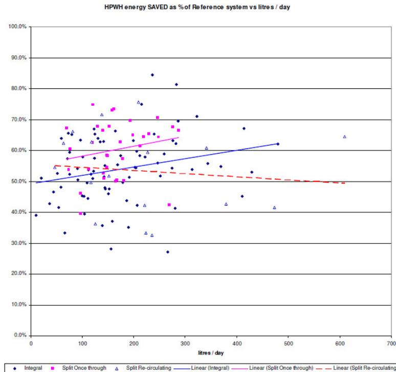
Fig. 22. Results of the EECA study of the performance of 127 heat pump water heaters considered to be well designed and installed.
