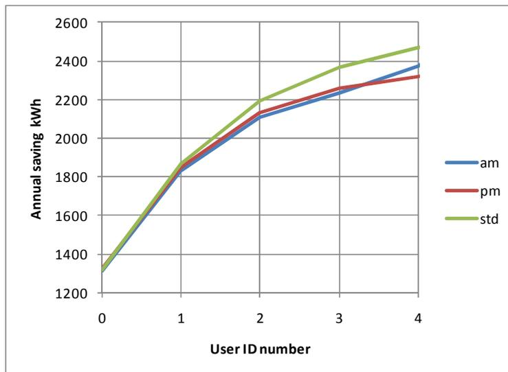
Fig. 2. Effect of different daily water use profiles on the annual kWh saving in purchased electricity using a solar water heater compared with the reference electric water heater. This figure applies to the North zone using a 2.4 m<sup>2</sup> solar collector (30 evacuated-tubes) and shows five levels of consumption (user 0 – 4).
