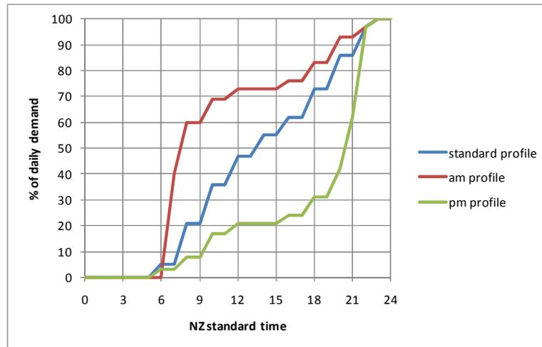
Fig. A1. Hot water demand profiles used in this study. The standard profile is defined in AS/NZS4234.
