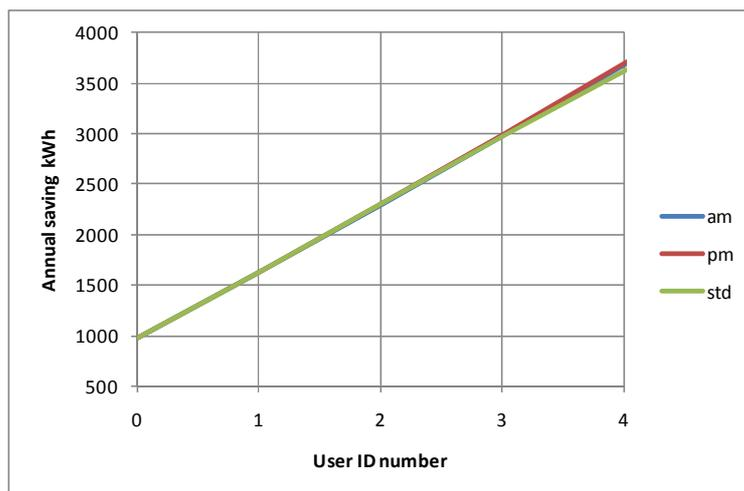
Fig. 4. Effect of different daily water use profiles on the annual kWh saving in purchased electricity for a heat pump water heater compared with the reference electric water heater. This figure applies to the North zone for five levels of consumption (user 0 – 4).
