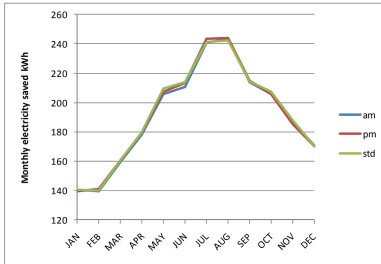
Fig. 3. Effect of different daily water use profiles on the saving in monthly purchased electricity for a medium level user in the North zone using the heat pump water heater.
