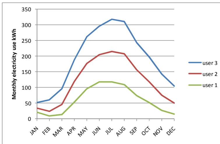
Fig. 6. Monthly electricity used by the representative solar water heater with a 2.4 m<sup>2</sup> collector (30 evacuated-tubes) in the North zone.
