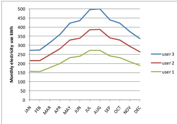
Fig. 5. Monthly kWh used by a reference electric water heater in the North zone.
