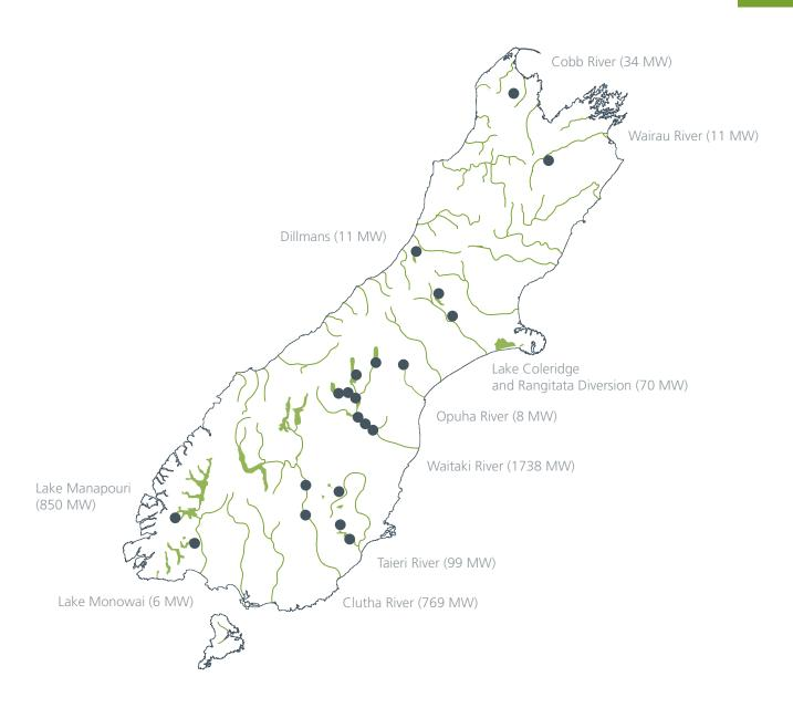
Figure 2.5 Installed hydroelectricity generation in the South Island. Each dot represents a power scheme larger than 5 MW.
