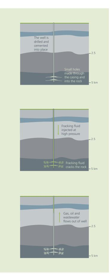
Figure 1.2 The main stages of cracking the rocks so oil and gas can flow.
