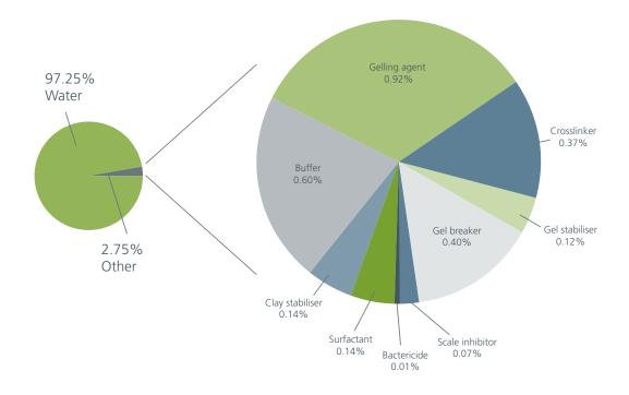
Figure A: A typical breakdown of the components of fracking fluids used in New Zealand. The data is taken from the assessments of environment effects in consent applications for Taranaki fracking operations since July 2011.
